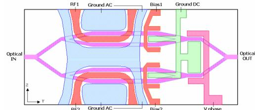
Figure 2. A LiNbO<sub>3</sub> X-cut QPSK modulator.
