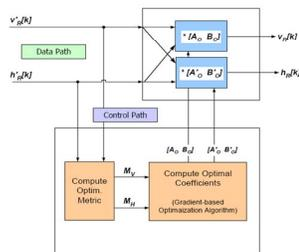
Figure 4. Schematics of the digital polarization rotator that is performed at the base-band
