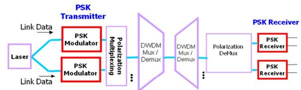
Figure 1. A typical coherent optical QPSK link.
