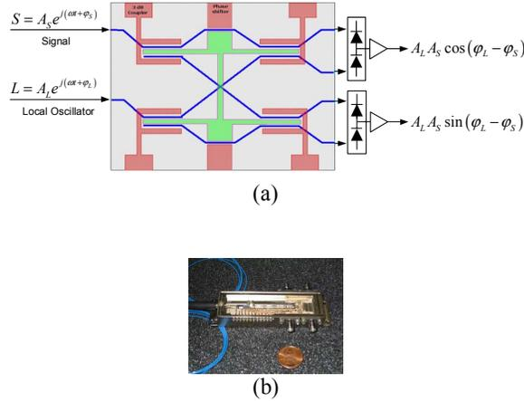
Figure 3. Coherent receiver. (a) Schematics of the receiver. The colored section is the 90° optical hybrid. (b) A package coherent receiver.
