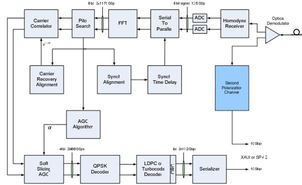
Figure 7. OFDM receiver DSP architecture.
