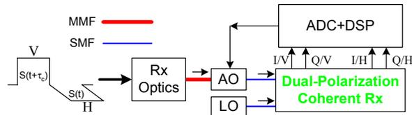
Figure 1. Block diagram of the proposed Rx. ADC: analog-to-digital converter.
