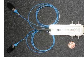
Figure 3. Photograph of the ICR. The ICR package has two input polarization-maintaining fibers for the received optical OFDM and the LO. Dimensions:  $127 \times 26 \times 13$  mm<sup>3</sup>.
