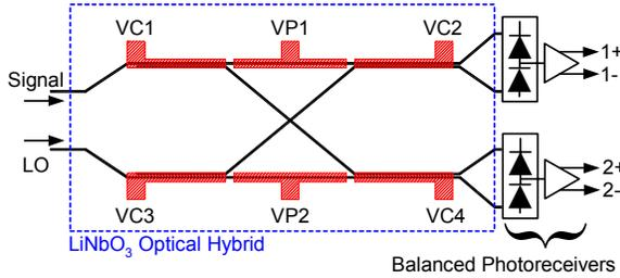
Figure 2. Schematic of an ICR with an optical hybrid and two sets of balanced photoreceivers. VC1 to VC4 are the coupler electrodes while VP1 and VP2 are the phase electrodes.
