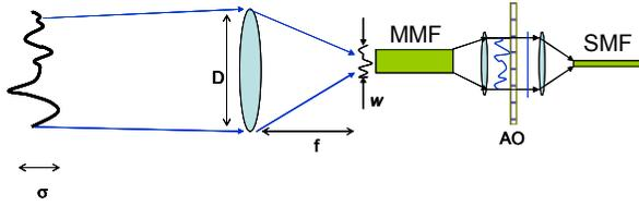
Figure 5. Schematic of the optical coupling stage of the proposed CLRR.
