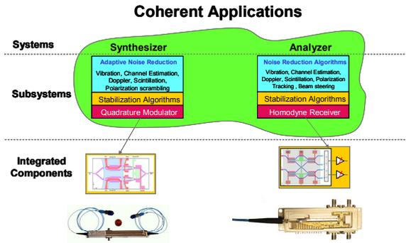
Figure 6. A unified layered architecture for fieldable digital coherent interferometric communications and sensing.
