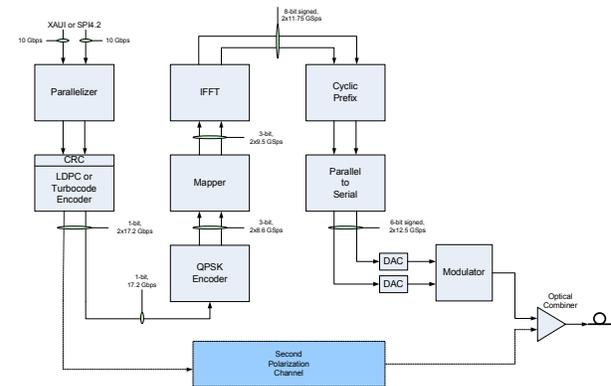
Figure 4. OFDM transmitter DSP architecture.
