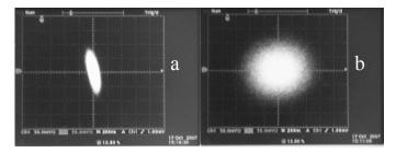
Fig. 4. Hybrid control with optical noise: a. initial constellation of received IQ signals, b. after control algorithm was run. OSNR 0.6 dB (RB: 0.01 nm).
