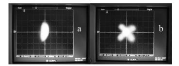
Fig. 5. Hybrid control with differential detection of RZ-QPSK: a. initial constellation of received IQ signals, b. after control algorithm was run.
