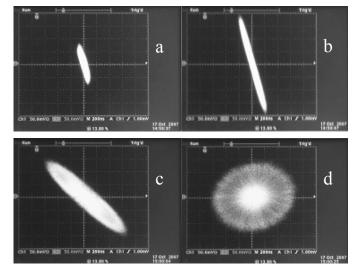
Fig. 3. Hybrid control with homodyne detection of RZ-QPSK: a. initial constellation of received IQ signals, b. after output couplers control iteration, c. after input couplers control iteration, d. after phase shifters control iteration. Displayed on a free-running oscilloscope.
