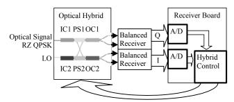
Fig. 1. Optical hybrid control path in the coherent receiver. Couplers: IC1, IC2, OC1, OC2; Phase Shifters: PS1, PS2.
