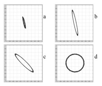
Fig. 2. Simulation of hybrid control: a. initial constellation of received IQ signals, b. after output couplers control iteration, c. after input couplers control iteration, d. after phase shifters control iteration.
