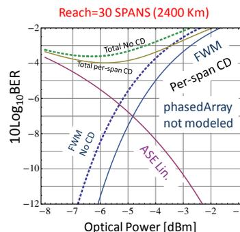
Fig. 2: BER performance for CD uncompensated link of 30 spans. Top plot is the total BER ( $10^{-4}$  at  $-5.5$  dBm), ignoring ASE (10<sup>-4</sup> at  $-1.5$  dBm). The substantial increase in the phased-array effect, while accounting for dispersive mismatch in each span.
