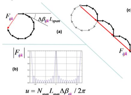
Fig. 1: Phasor addition of the FWM contributions of the multiple spans (a): CD uncompensated link (b): Array Factor plot. (c): Link with periodic compensation every few spans. Here the phased-array amplitude reduction is less favorable.
