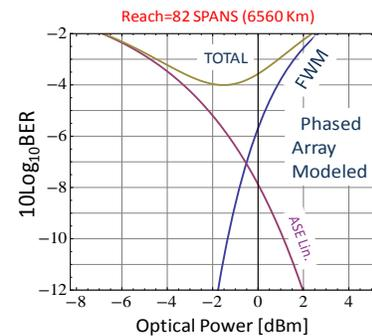
Fig. 3: BER performance for CD uncompensated link of 82 spans. Top plot is total BER ( $10^{-4}$  at  $-1.5$  dBm). The substantial increase in the phased-array effect, while accounting for dispersive mismatch in each span.
